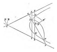
P'PN the line in which their plane is cut by a circular section GPK or gP'k.
